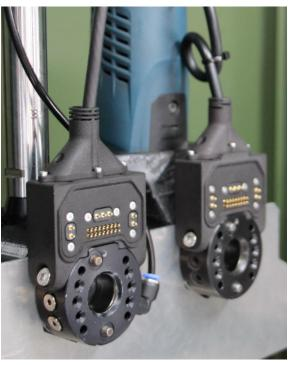
Although both High Yield PA11 and PA12 are suitable for connectors, SAF™ PA12 was applicable in this specific instance as it exhibits improved stiffness and accuracy. In comparison, PA11 has excellent impact toughness and ductility for applications that experience more dynamic loads.
